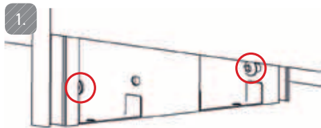
FIG. 3: Loosen screws on both legs of the convector body and remove the top cover. (do not remove the screws completely!!!).
