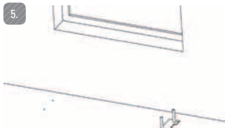
FIG. 7: Install the supply and return pipes in the floor and drill the holes for attaching the convector to the floor.
