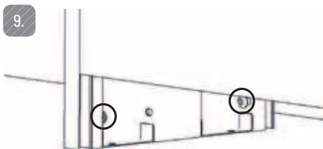
FIG. 11: Tighten the screws on convector legs.
